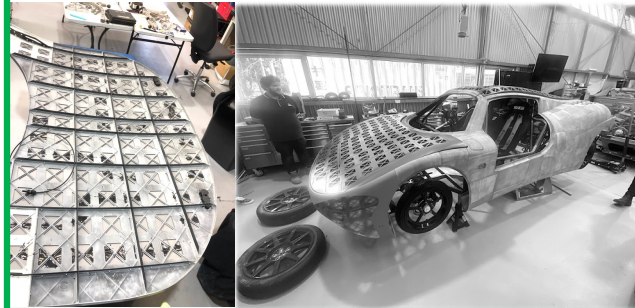
MJF printed external panel housing the solar arrays of the solar car
